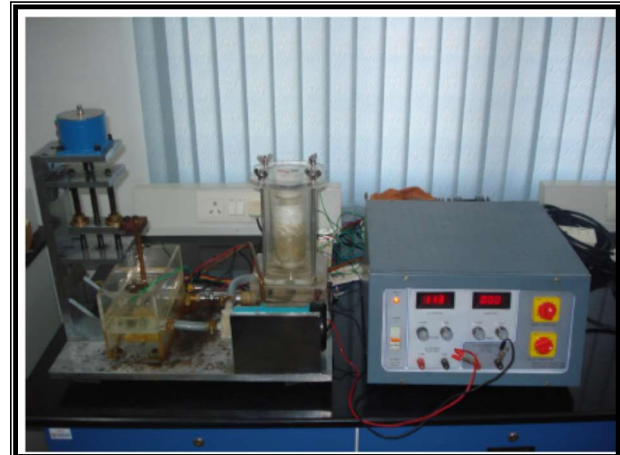
Figure 3.1: Experimental lab view setup of Micro Electric Discharge Machining
