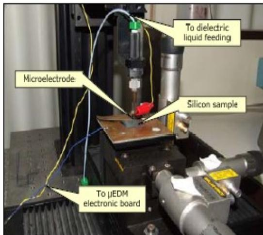
Figure:-1.2 Micro EDM machine with the Pt-Ir microelectrode, XYZ piezoelectric actuators and XY-Z micrometric translation stage (PTFE vat removed).
