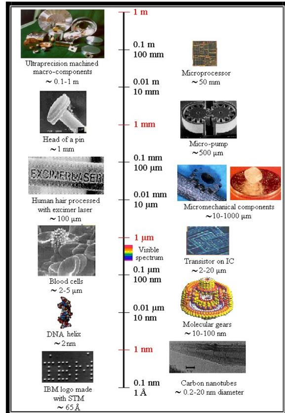
Figure: - 1.1 Size scale and examples of micro- and nano components.
