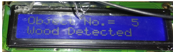
Figure 13: LCD showing object count with wood detection
