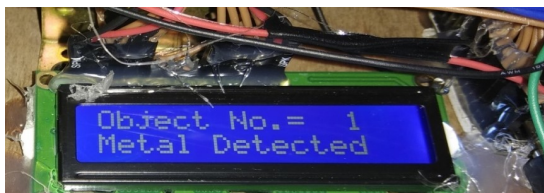
Figure 14: LCD showing object count with metal detection
