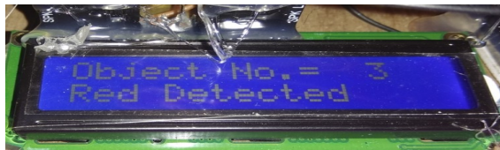
Figure 12: LCD showing object count with color detection (Red)
